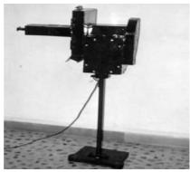
Fig. 7: Power operated banana slicer (Sonawane et al., 2011)
