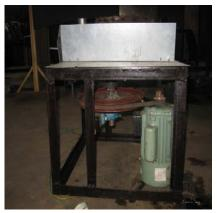
Fig. 6: Motorized plantain slicer (Adewumi et al., 2011)
