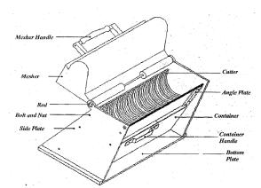
Fig.5:Mechanized plantain slicer (Obeng, 2004)
