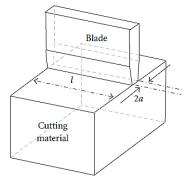
**Fig. 2:Interaction between the blade and the material while cutting** (Zhou et al., 2006)
